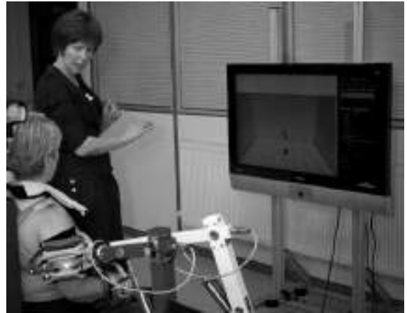
Figure 26.4 iPAM: A physiotherapist instructing the patient on how to use the stroke rehabilitation robotic system for arm exercises. Reproduced with permission of iPAM team, Leeds University, UK.
