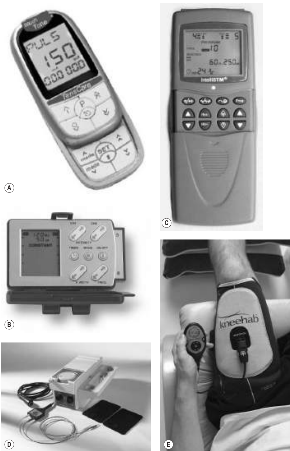
Figure 19.15 (a–c) Battery-powered (portable) muscle stimulators, all of which will deliver muscle-stimulating currents: (a) NMES stimulator (TensCare); (b) NMES stimulator (Body Clock); (c) IntelliSTIM (Natures Gate); (d) multimodal mains-powered device – part of MediLink (EMS Physio); (e) stimulator with dedicated knee sleeve electrode system (BMR Neurotech).
